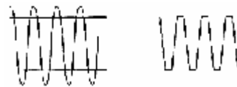
High gain causes wave to clip
